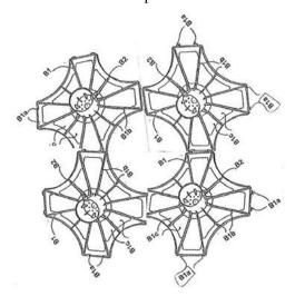
where it can be seen how the four feet at the base of the invention, installed and ready to accommodate the columns, are directly hooked together by means of connecting devices located at the ends of the short arms (where the 'arms' are the extensions of the foot from its centre outwards).
